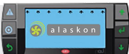
The controller start up screen can be customised to the customer's design to display any requirement. For example: time, date, customer web address etc
